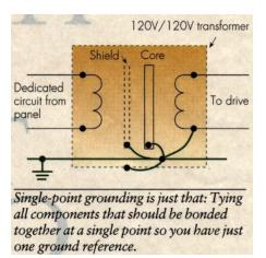
This prompted us to check the wiring of the shielded isolation transformers. Proper wiring for this installation, shown in the diagram above, requires the incoming ground, shield, core, and secondary neutral and ground all to bond at one point. This configuration is a *single-point ground*.
